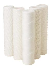
Pentair<sup>‡</sup> Pentek<sup>‡</sup> CW Series Cartridges are manufactured from a durable polypropylene cord that is wound around a rigid polypropylene core. They are an economical solution to reduce fine sediment, including sand, silt, rust and scale particles.
